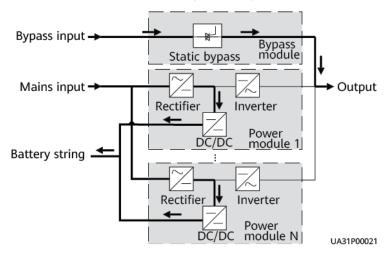
Figure 1-6 UPS conceptual diagram in bypass mode
