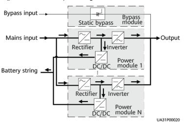
Figure 1-5 UPS conceptual diagram in normal mode
