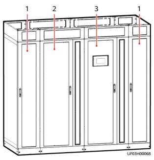
Figure 2-8 UPS + bottom cabling cabinet
