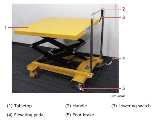
Figure A-1 Lifting trolley
