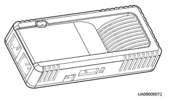
The RS485 communications port of the T/H sensor is an RJ11 (6P6C) port. If multiple T/H sensors need to be cascaded, connect the RJ11 port on each T/H sensor.
