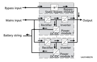
Figure 1-8 UPS conceptual diagram in S-ECO mode
