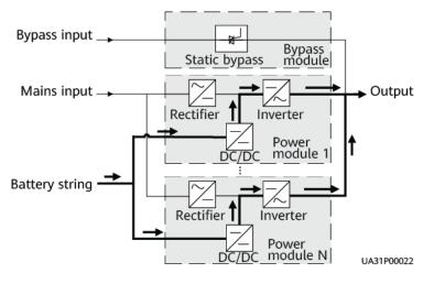
Figure 1-7 UPS conceptual diagram in battery mode
