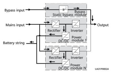
Figure 1-9 UPS conceptual diagram in ECO mode
