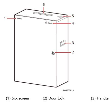
(4) Huawei logo (5) Signal cable outlet (6) Power cable outlets
